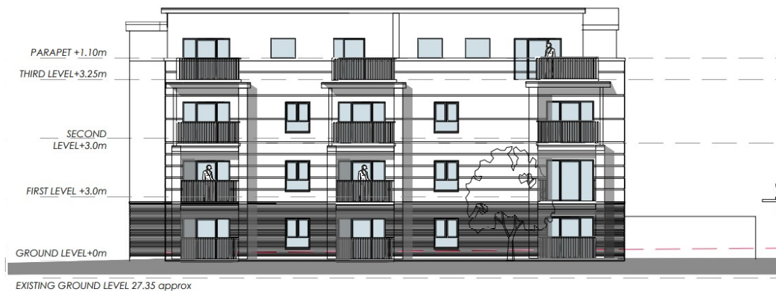
REAR ELEVATION ( Rail line Side)
